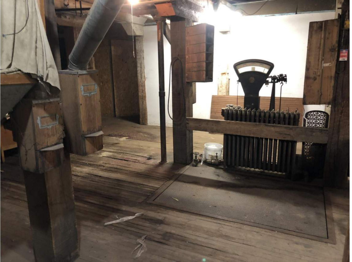
FIGURE 7 - DUCTS AND SEED DISPENSING DEVICES ON THE FIRST FLOOR DIRECTLY BELOW THE MULTI-STORY GRAIN BINS; THE SEED WOULD BE COLLECTED FROM THE DISPENSERS AND THEN PLACED ON THE SCALE SET IN THE FLOOR.
