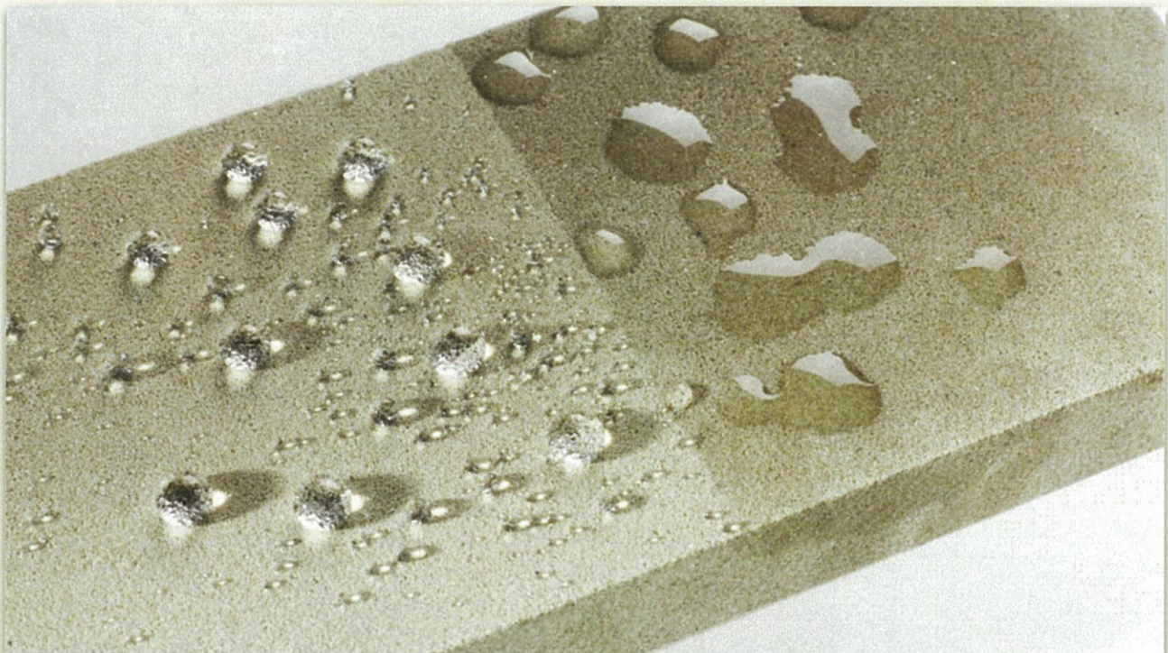
Left side: excellent water-beading effect after Protectosil® treatment, right side: without treatment
