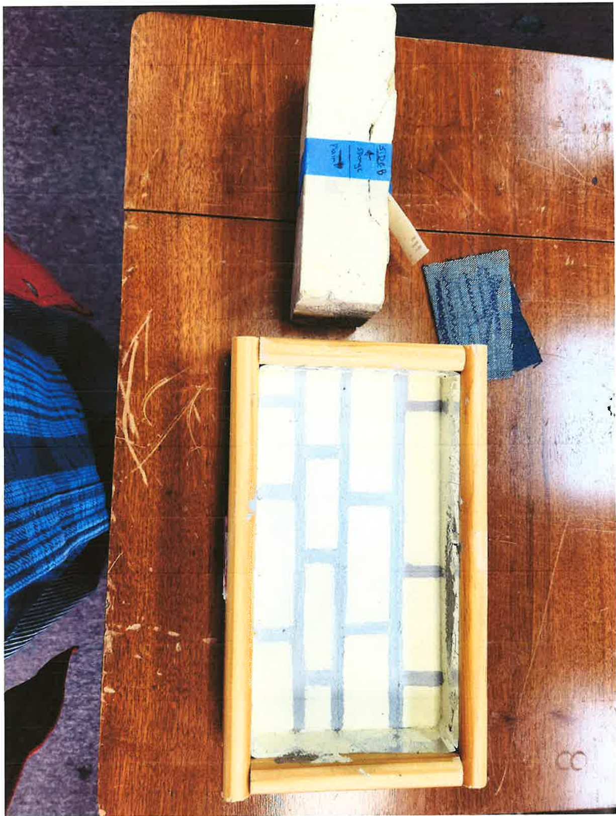
Sample Painted Concrete with Mortar & Painted Block (Overhead View)
