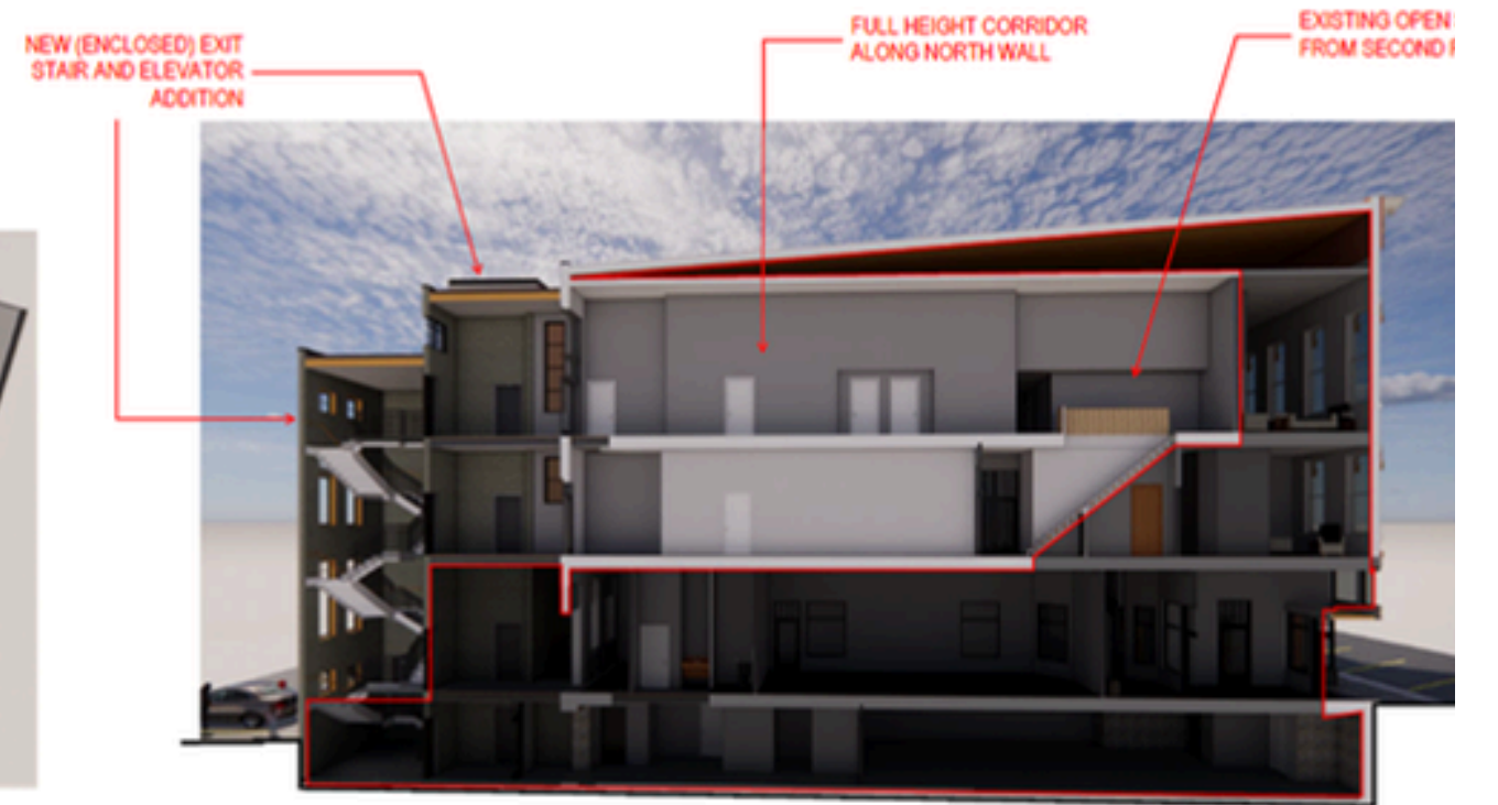
SECTION THRU BLDG LOOKING NORTH
