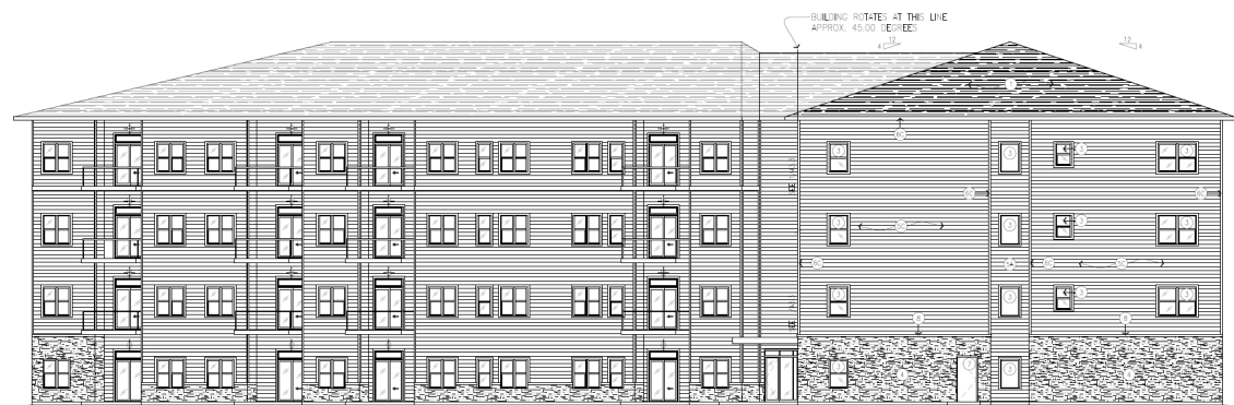
5 SOUTHWEST EXTERIOR ELEVATION ORIGINAL SCALE: 1/8" = 1'-0"
