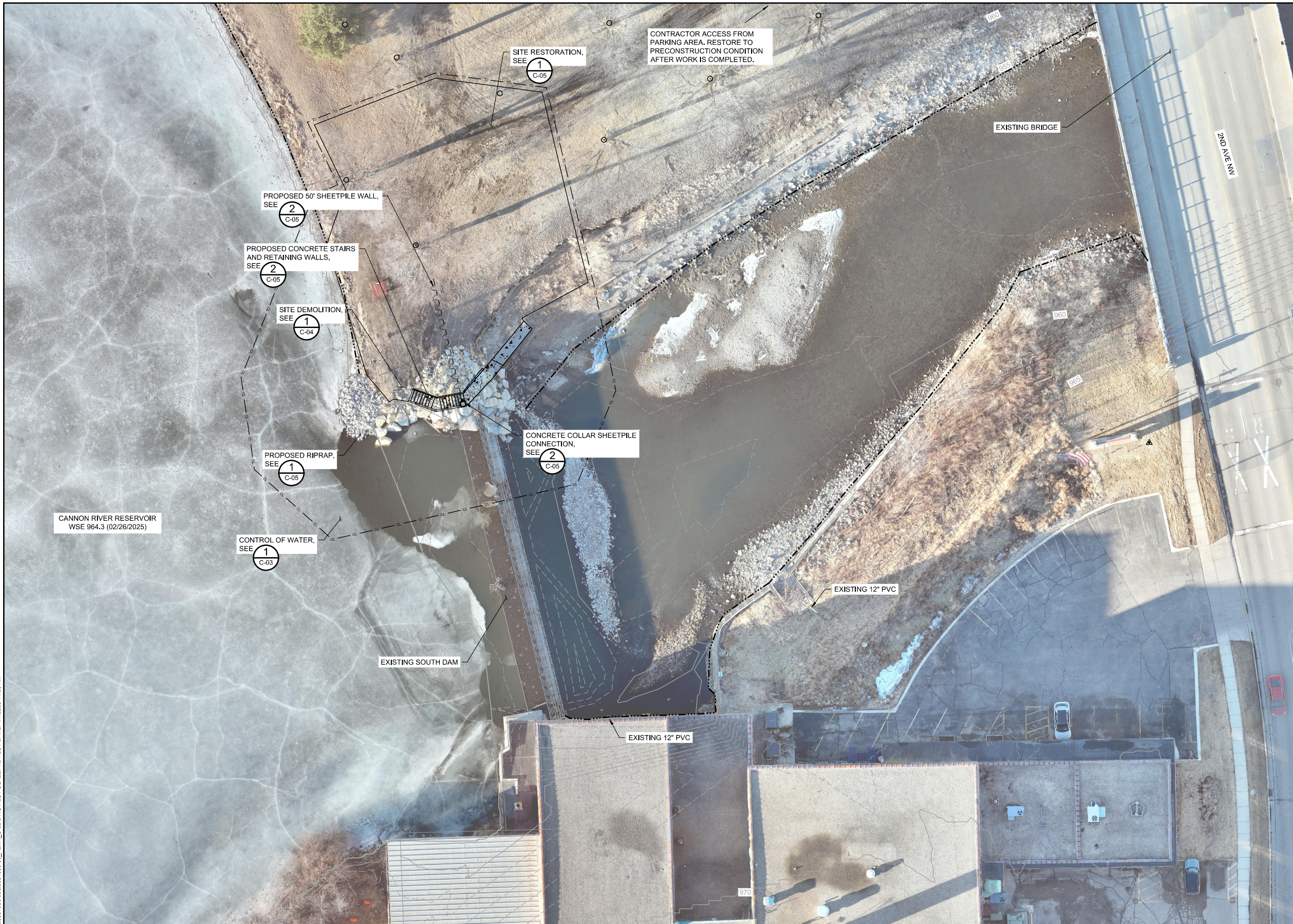
1 PLAN: SOUTH SPILLWAY SITE MODIFICATIONS
