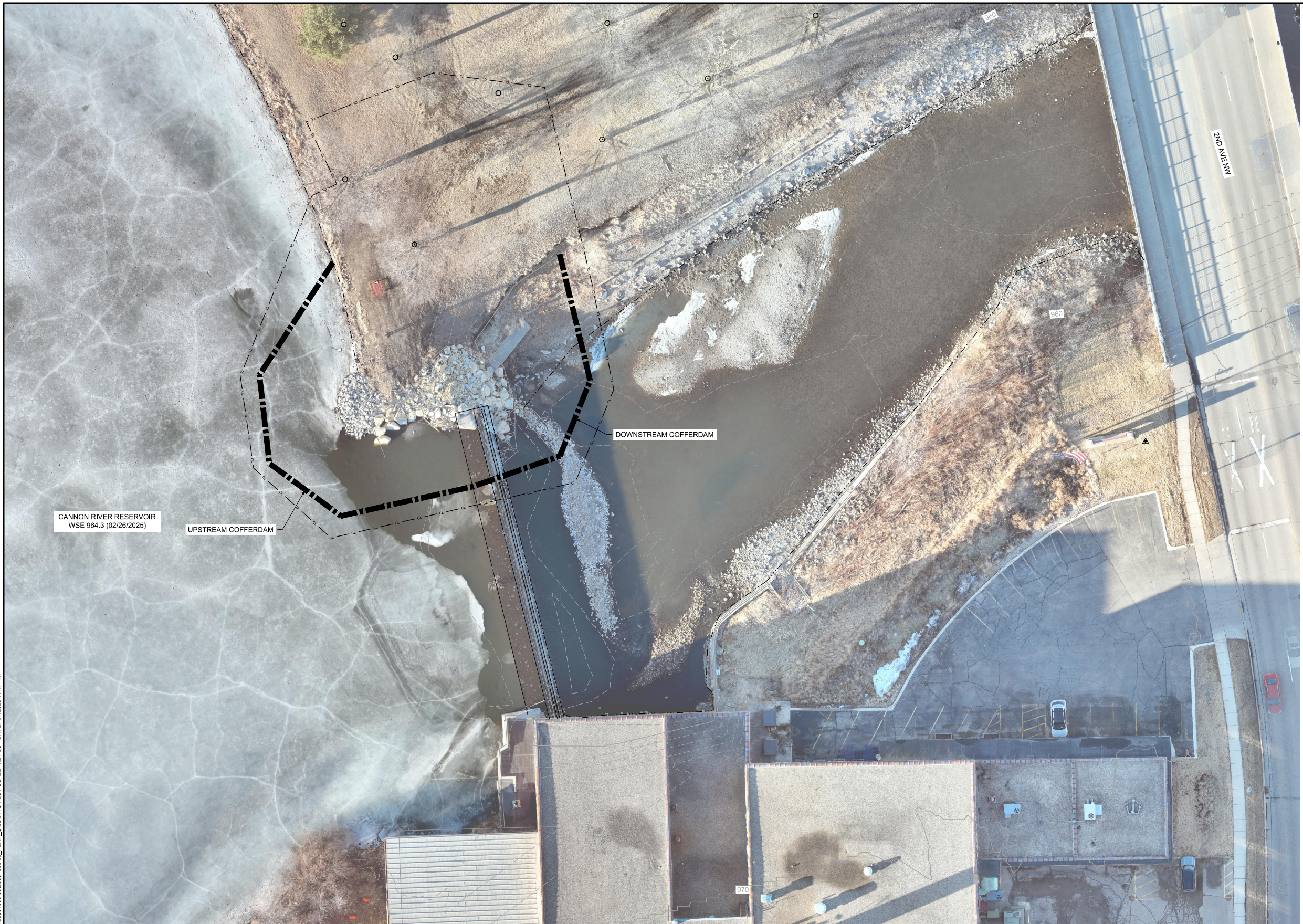
1 PLAN: SOUTH SPILLWAY WATER CONTROL
