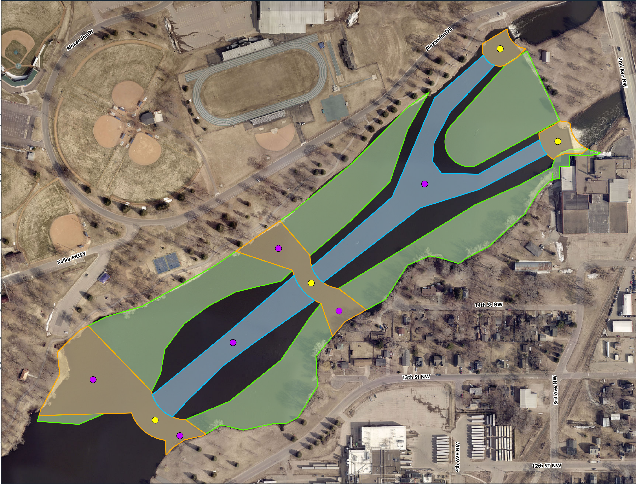
Proposed Boring Locations Woolen Mill Dam Fairbault, MN FIGURE 1 BARR
